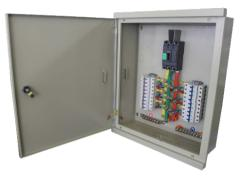
Type: MG-M408C [Ue] rated operational voltage: 415VAC Breaking capacity: 10kA Rated current: 100A Rated frequency: 50/60Hz Protection type: overload protection, short-circuit protection Rated impulse withstand voltage: 6kV Degree of protection: IP54 Feed: Top and bottom Out door, Installation: Flush mounted Material: Steel Board Dimension: 500x600x180mm Enclosure color: Light Gray Standard: IEC60947-1 IEC60947-2
